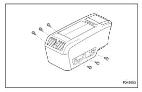
(b) Keeping the rear console box pulled in the rear direction of the vehicle, install the 6 bolts to the left and right sides.
