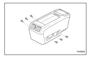
(b) Keeping the rear console box pulled in the rear direction of the vehicle, remove the 6 bolts from the left and right sides.
