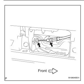
(c) Connect the console box lock control cable assembly and install the rear console box.
