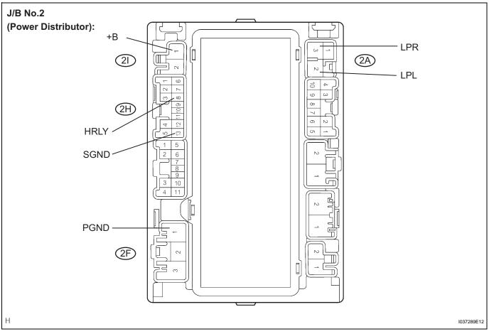
Connect the positive battery lead to terminal +B of the J/B No.2 and the negative lead to terminal SGND, PGND.
