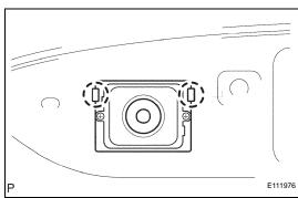
(b) Disengage the 2 claws and remove the television camera.
