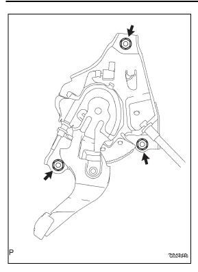
(e) Remove the 3 nuts and parking brake control pedal assembly.
