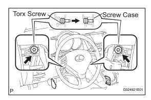
(b) Pull out the horn button assembly from the steering wheel and disconnect the airbag connector.
