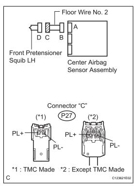
(a) Disconnect the connector from the center airbag sensor assembly.
