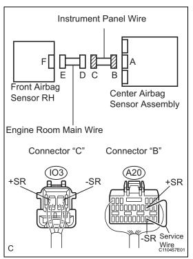
(a) Disconnect the instrument panel wire connector from the engine room main wire.
