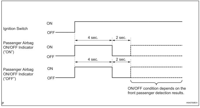
When the front passenger occupant classification system has trouble, both the SRS warning light and the passenger airbag ON/OFF indicator come on. In this case, check the DTCs in the "AIRBAG SYSTEM" first. Then troubleshoot the occupant classification system if DTC B1150/23 is detected and troubleshoot the passenger airbag ON/OFF indicator if DTC B1152/28 is detected.
