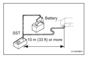
(2) Connect the SST connector to the driver side knee airbag assembly.
