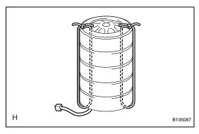
Position the curtain shield airbag assembly inside the tire as shown in the illustration.
