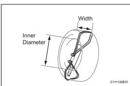
(3) Position the front seat side airbag assembly inside the tire as shown in the illustration.
