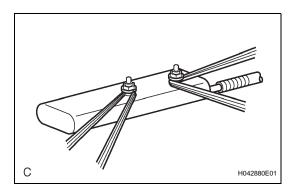
(2) Wind the wire harness around each of the stud bolts of the front seat side airbag assembly as shown in the illustration.
