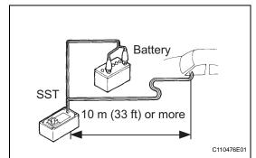
(2) Connect the SST connector to the front seat side airbag assembly connector.
