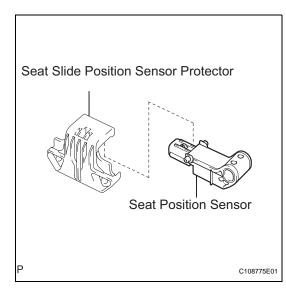
(b) Using a "torx" socket wrench (T30), remove the "torx" screw and the seat position sensor.
