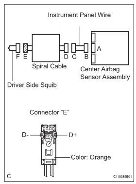
(a) Measure the voltage according to the value(s) in the table below.
