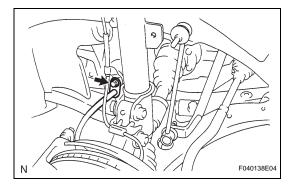
(d) Install the front flexible hose No. 1 and speed sensor wire harness front LH with the bolt.
