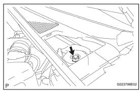
(e) Fully tighten the lock nut.
