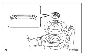
(g) Install a new front suspension support bearing LH.
