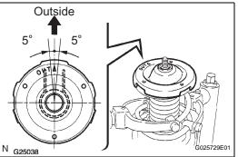
(f) Install the front coil spring seat upper LH to the shock absorber assembly front LH with the mark facing to the outside of the vehicle.
