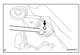
(d) Remove the bolt, nut and strut rod from the rear axle carrier.
