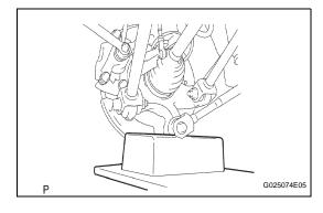
(b) Remove the bolt and nut, and separate the parking brake cable.
