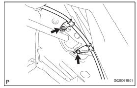
(c) Remove the bolt and nut, and disconnect the strut rod (front side).
