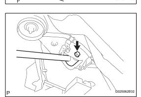
(c) Connect the strut rod (inner side) with the bolt and nut.
