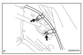
(c) Install the parking brake cable with the bolt and nut.
