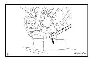
3. FULLY TIGHTEN STRUT ROD ASSEMBLY REAR
