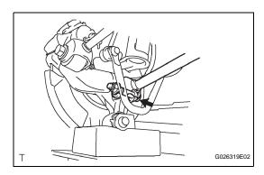
(b) Connect the rear suspension arm assembly No. 1 (outer side) to the rear axle carrier with the bolt and nut, and temporarily tighten the bolt and nut.
