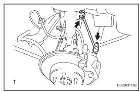
Check that neither crack nor grease leakage exists on the dust cover.
