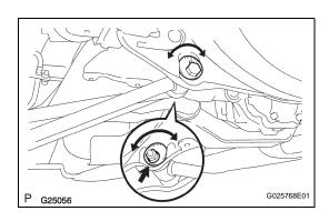
(b) Turn the adjust cams by an equal amount to adjust toe-in.
