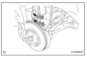
(c) Remove the 2 nuts and bolt on the lower side of front shock absorber with coil spring.
