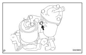
(c) Remove the bolt and the height control dryer assembly from the height control compressor assembly.
