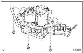
(b) Install the rear height control compressor bracket with the 3 bolts onto the height control compressor bracket.
