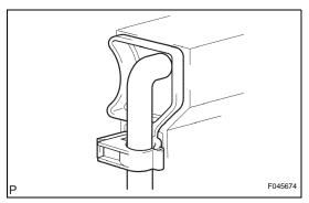
(c) Connect the hose to the cap grommet and clamp it.
