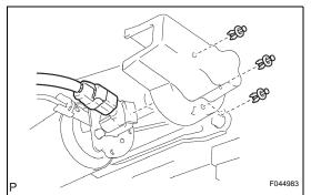
(f) Using SST, disconnect the tube from the pneumatic w/ tube tank assembly.
