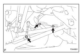
(b) Remove the torx nut, the 2 nuts and the height control sensor RR LH from the vehicle.
