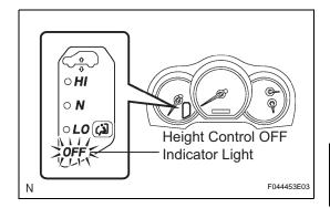
(5) Check that the height control OFF indicator light comes on and goes off at 0.125 second intervals. (4 Hz)
