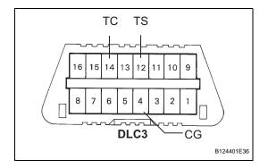
(7) Using the SST(s), connect the 3rd terminal of the SST to terminal TC in the DLC3.SST 09843-18040
