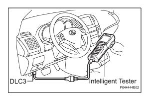
(5) After completing the check, remove the SST(s) from DLC3.
