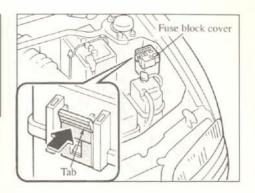
If the headlights orother electrical components don't work and the fuses in the cabin are OK, inspect the fuse block under the hood. If a fuse is blown, it must be replaced. Follow these steps:
