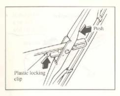
Raise the wiper arm and turn the blade assembly to expose the plastic locking clip.
