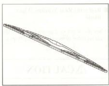
3. Install a new blade in the reverse order of removal.
