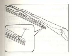
4. Carefully insert the new blade rubber. Then install the blade assembly in the reverse order of removal.
