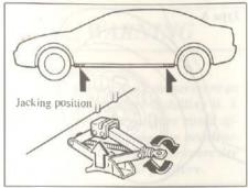
8. Place the jack under the side sill at the front or rear jacking position closest to the tire being changed.
