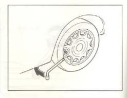
6. Pry off the center cap with the beveled end of the lug wrench.
