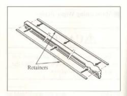
Remove the metal retainers from the blade rubber and install them in new blades.
