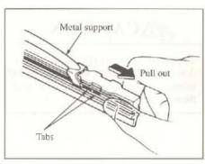
2. Hold the end of the rubber and pull until the tabs are free of the metal support.
