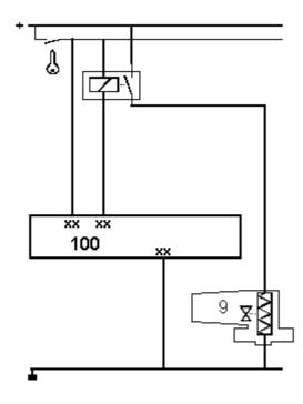
The auxiliary air valve has a connector with two terminals. One of those terminals is continuously connected with ground. The other terminal is connected with a relay switching the power to the heating element.
