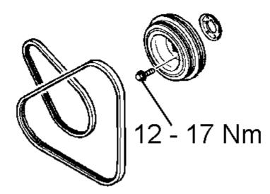
Fit the ancillary drive belt Refit the engine lower covers
