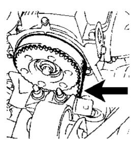
The tension is set at a deflection of: Refit the timing belt guide plates 5.5 - 6.5 mm
