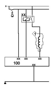
The electrical behaviour of an injector is determined by the coil inside. As a current flows through the coil the injector needle is pulled up against the spring force which courses the fuel to be injected. Two types of injector coils are used. The resistance of a normal coil is approximate 15 ohms. Other injection systems use low resistance coils (approximate 1-2,5 ohms).
