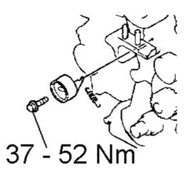
Push the tensioner pulley away from the timing belt
