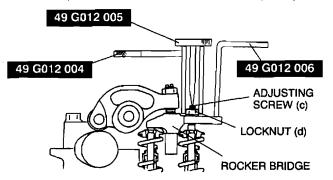
(3) Loosen the rocker arm locknut (b) using the SST (49 G012 004), and then turn the adjusting screw (a) using the SST (49 G012 005) until it is separated from the rocker bridge completely.
