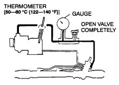
8. Remove the gauge set. Install and tighten the pressure pipe to the specified torque.
