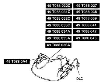
Listen to the double beep. The NGS tester is now initialized. Begin the powertrain control system functional test.
