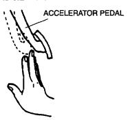
Move the idle switch with the accelerator pedal as described in Step 2, and install a locknut where there is continuity in the idle switch.
