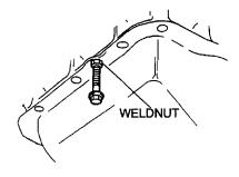
4. Using a separator tool, separate the oil pan.
