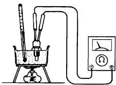
4. Measure the resistance between ECT sensor terminal C and body ground using an ohmmeter.
