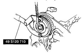
3. Remove the camshaft pulley using the SST.
