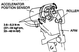
4. If as specified, perform "IDLE SWITCH ADJUSTMENT". If not as specified, perform "ACCELERATOR POSITION SENSOR INSPECTION". (Refer to CONTROL SYSTEM, ACCELERATOR POSITION SENSOR INSPECTION.)
