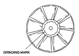
3. If there are damaged fins, cracks or bends, replace the turbocharger. (Refer to EXHAUST SYSTEM, EXHAUST SYSTEM REMOVAL/INSTALLATION.)
