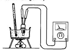
Measure the resistance of the IAT sensor using an ohmmeter.
