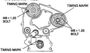
7. If not, align all timing marks according to the procedure below.
