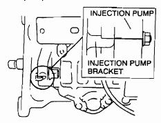
2. Tighten the bolts and nuts in the order shown.
