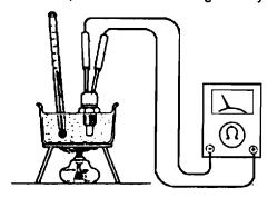
Measure the resistance between the engine coolant temperature sensor terminals A and B using an ohmmeter.
