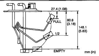
If not as specified, replace the fuel gauge sender unit.
