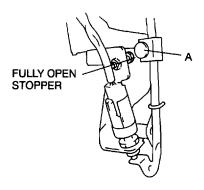
2. Confirm that the voltage of the PCM 2F terminal (accelerator position sensor) is within specification.
