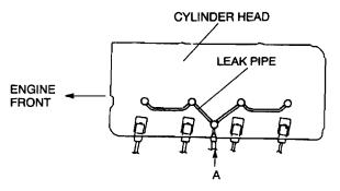
2. Apply soapy water to the joint area of the leak pipe and the injection nozzle, and verify that there is no leakage.
