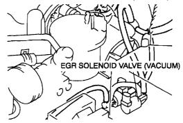
3. Inspect for airflow between each port under the following condition.
