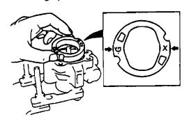
2. Install the vanes in the rotor with the rounded edges outward.
