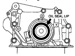
2. Remove the oil seal using a screwdriver protected with a rag.
