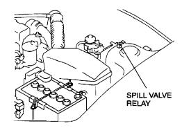
3. Inspect for continuity between terminals of the relay using an ohmmeter.
