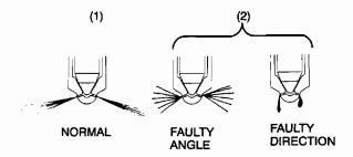
4. If the atomization condition is not within the specification, replace the injection nozzle.
