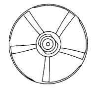
If there are damaged fins, cracks or bends, replace the turbocharger. (Refer to EXHAUST SYSTEM, EXHAUST SYSTEM REMOVAL/INSTALLATION.)
