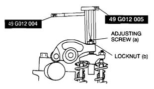
(4) Insert a feeler gauge between the rocker arm and rocker bridge (e).
