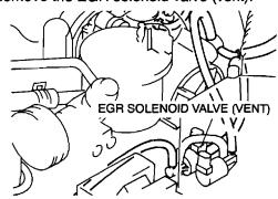
3. Inspect for airflow between each port under the following condition.
