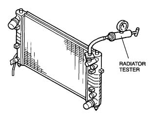
(6) Put the radiator into water slowly with the radiator tester connected.
