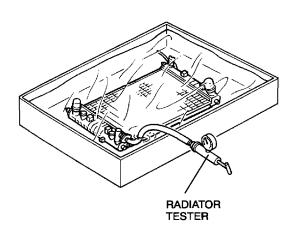
(7) Inspect for air leakage.
