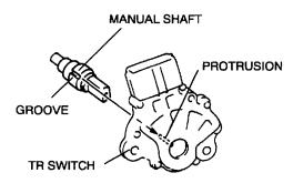
Turn the TR switch so that the neutral hole is in line with the flat, straight surfaces on either side of the manual shaft.
