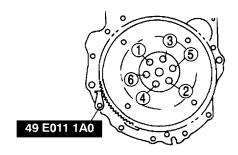
2. Remove the drive plate mounting bolts.
