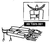
If clearance B is more than the specification, reduce clearance A of the SST and crimp the band again.
