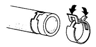
4. Verify that the hose clamp does not interfere with any other components.
