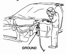
4. Cover the peripheral parts of the welding area to protect them from weld spatter.
