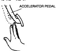
3. Move the idle switch with the accelerator pedal as described in Step 2, and install a locknut where there is continuity in the idle switch.
