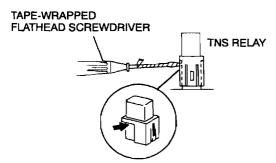
2. Pull out the TNS relay while pressing the flathead screwdriver downward.
