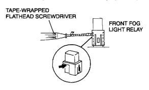
2. Pull out the front fog light relay while pressing the flathead screwdriver downward.
