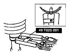
3. If clearance B is more than the specification, reduce clearance A of the **SST** and crimp the boot again.
