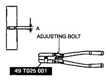
2. Crimp the wheel side small boot band using the **SST**. Verify that clearance B is within the specification.
