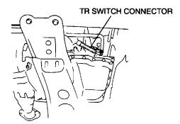
Remove the clip and disconnect the selector cable.
