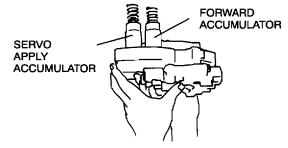
2. Install the control valve body component.
