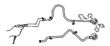
2. Align the marks, and slide the oil hose onto the oil pipe until it is fully seated as shown.
