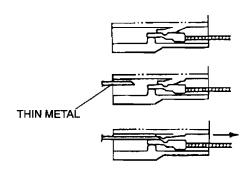
2. Pull the terminal out of the connector.
