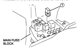
Front fog light relay See T-22 Front fog light relay removal note
