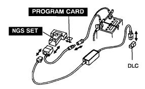
2. Select the "DIAGNOSTIC SUPPORT PROCEDURE" on the NGS. (See F1-34 ON-BOARD DIAGNOSTIC TEST, Diagnostic Support Procedure.)
