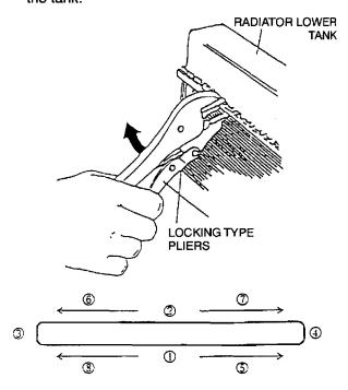
5. Verify the height of the header tabs is same as the height before removal.
