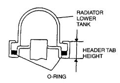
2. Insert the end of a medium tip screwdriver between the end of the header tab and the outer tank.
