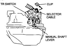
6. Remove the manual shaft nut, washer and manual shaft lever.
