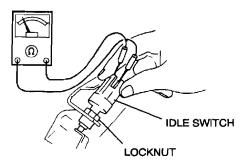
4. Press the accelerator pedal gradually by hand and verify that the output voltage of the PCM 2F terminal (accelerator position sensor) is within the specification when the output voltage of the PCM 1T terminal (idle switch) changes to B+ from below 1.0 V.
