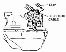
Rotate the manual shaft to the converter housing side fully, then return 2 notches to set the N position.
