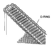
Position the radiator tank in the original direction to the core using care not to scratch the tank sealing surface with the header tabs.
