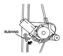
Slowly insert the reset jig into the hole where the bushing was installed until it stops.
