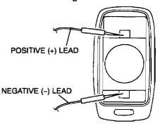
While pressing the battery as shown in the figure, press the LOCK and UNLOCK buttons on the transmitter at the same time for 5 seconds.
