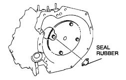
Using a flathead screwdriver to prevent the drive plate from rotating, remove the torque converter nuts.
