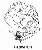
7. Loosen the TR switch mounting bolts.
