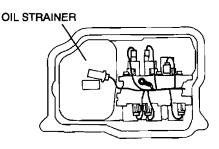
Remove the control valve body installation bolts A as shown, then remove the control valve body component as shown.
