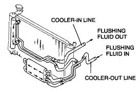
2. Flush oil cooler/lines until discharge fluid is clean.
