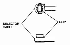
14. Connect the selector cable to the manual shaft lever as shown in the figure.
