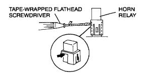
2. Pull out the horn relay while pressing the flathead screwdriver downward.
