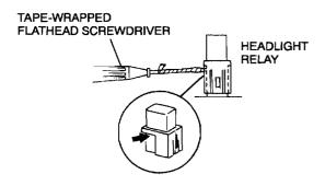
2. Pull out the headlight relay while pressing the flathead screwdriver downward.
