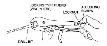
Squeeze the header tabs down in order as shown against the lip of radiator outer tank base with locking-type pliers while rotating the pliers toward the tank.
