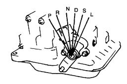
2. Install the selector cable to the selector lever.
