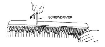
Remove the radiator outer tank and O-ring (gasket) from the core header when all of the tabs are opened.
