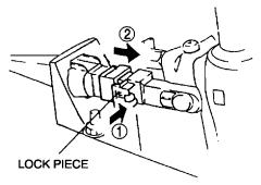
8. Shift the selector lever from P position to L range, and make sure that other components that area to there is no interfere the lever.
