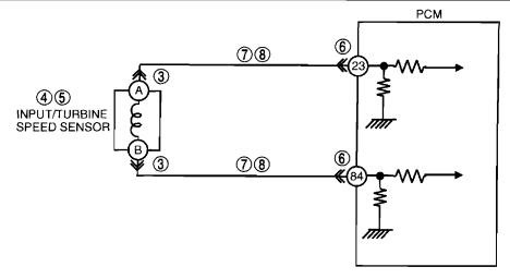
INPUT/TURBINE SPEED SENSOR
