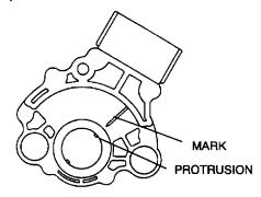
10. Install the TR switch while aligning the protrusion and groove as shown.
