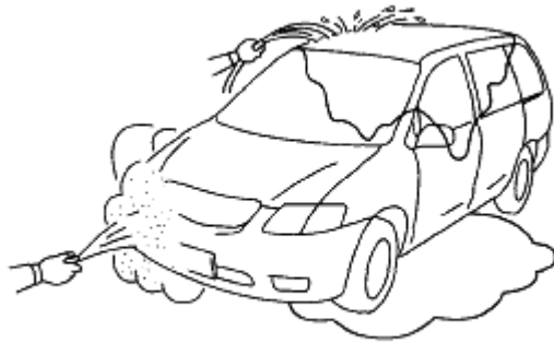
Fig. 9: Spraying Water Onto Vehicle Courtesy of MAZDA MOTORS CORP.
