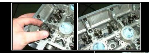
Follow the same procedure as above to adjust the next cylinder. When adjustment is correct, mark both rocker arms with a black "sharpie" marker indicating their appropriate location.
