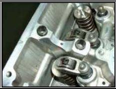
Note: it's important to keep each rocker with the lobe that it was adjusted for. Often manufacturing tolerances in the cylinder head and on the camshaft are different for each lobe.
