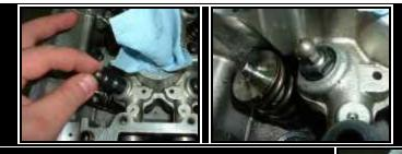
Install rocker arms on 1 set of valves (for example both exhaust valves on cylinder number 1)
