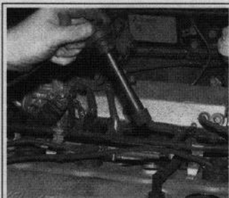
Fig. 90 Carefully twist the boot end of the spark plug wire and withdraw the spark plug wire boot from the cylinder head
