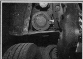
Fig. 52 The EVAP canister is typically located inside of the fender on most models covered by this manual
