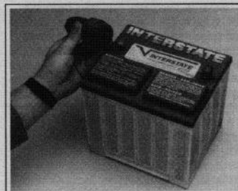
Fig. 58 The underside of this special battery tool has a wire brush to clean post terminals
