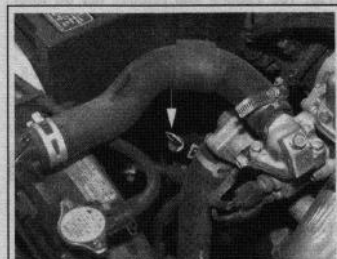
Fig. 168 The automatic transaxle dipstick is typically located under the air cleaner inlet tube. Pull the dipstick up to remove it from the transaxle
