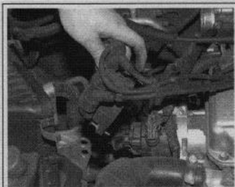
Fig. 106 . . . then remove the cap from the distributor
