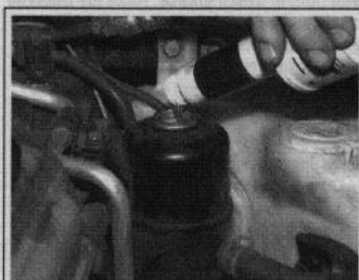
Fig. 218 If the power steering level is low, add fluid to the reservoir until the proper level is reached
