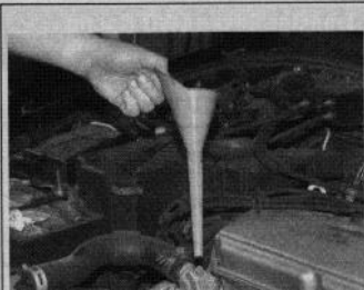
93151p84 Fig. 175 A long, thin funnel is necessary to access the transaxle dipstick tube
