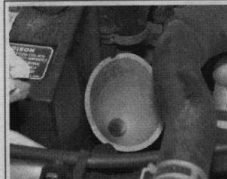
93151p83 Fig. 176 Place the funnel into the opening on the dipstick tube
