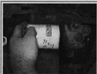
Fig. 158 When the filter is sufficiently loosened with the filter wrench, turn the filter by hand, but be careful, as oil will start to run out of the filter
