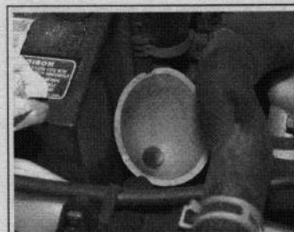
93151p49 Fig. 177 Pour the fluid directly into the funnel, periodically checking the fluid level to make sure you do not overfill the transaxle
