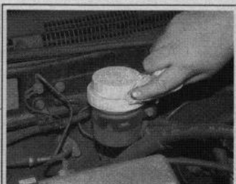
Fig. 207 Wipe the master cylinder reservoir clean before opening the cap to ensure that no contamination enters the brake fluid
