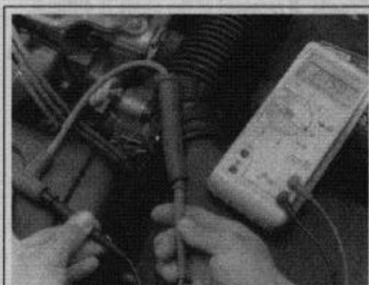
Fig. 102 Checking individual plug wire resistance with a digital ohmmeter
