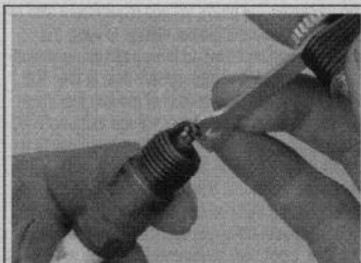
Fig. 99 Adjusting the spark plug gap
