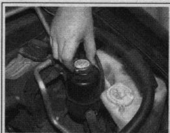
Fig. 215 Twist the reservoir cap, then lift up on the integral cap/dipstick assembly
