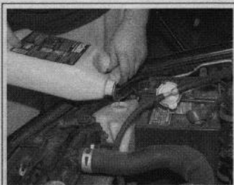
Fig. 204 . . . make sure to fill the coolant recovery tank to the proper level also
