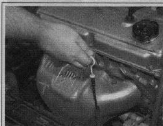
Fig. 149 Grasp the oil level dipstick and pull upward to remove it from the dipstick tube
