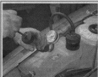
Fig. 194 Pump the cooling system with pressure, making sure not to overpressurize the system or damage can occur
