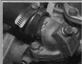
Fig. 190 A visual inspection for leaks will sometimes find a leak. This photo shows evidence of a leak at the upper radiator hose-to-thermostat housing junction
