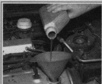
Fig. 163 . . . then insert a funnel, and pour oil directly into the engine
