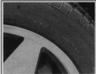
Fig. 138 Unidirectional tires are identifiable by sidewall arrows and/or the word "rotation"
