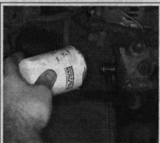
Fig. 159 Once the oil filter is completely unthreaded, remove the filter from the engine
