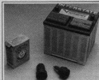
Fig. 57 Maintenance is performed with household items and with special tools like this post cleaner
