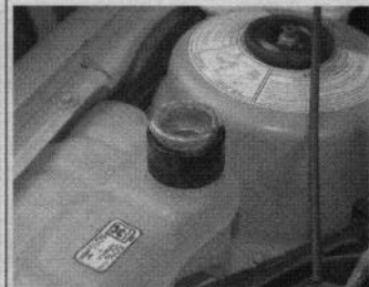
Fig. 193 Thread the adapter onto the recovery tank
