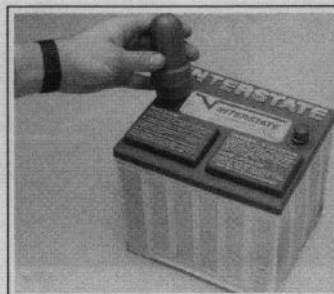
Fig. 59 Place the tool over the battery posts and twist to clean until the metal is shiny
