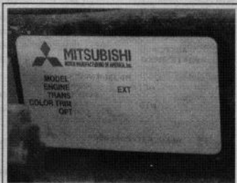
Fig. 33 The vehicle model, engine model, transaxle model, and body color code are all noted on the vehicle information code plate
