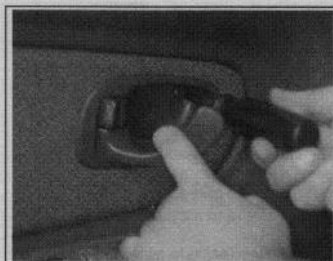
Fig. 42 Remove the inside pull handle retaining screw cover . . .
