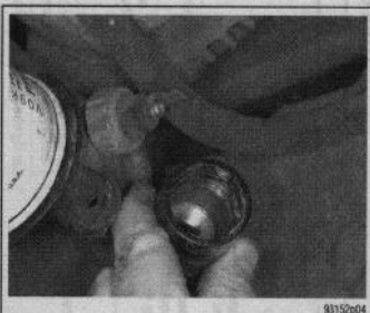
Fig. 62 . . . and the use of an oil pressure sending unit socket greatly aids the removal and installation
