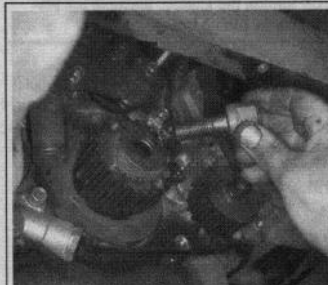
Fig. 175 Remove the bolt and remove the crankshaft timing belt pulley
