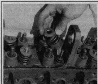
Fig. 248 Remove the valve spring and retainers from the cylinder head
