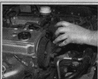
Fig. 8 . . . then carefully remove the cover from the engine
