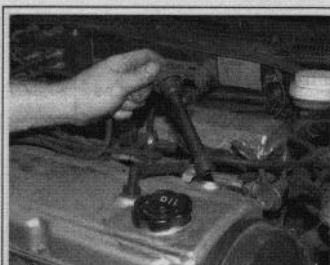
Fig. 5 Twist each spark plug wire to remove it from the spark plug . . .
