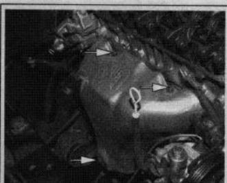
Fig. 66 Remove the heat shield retaining bolts . . .
