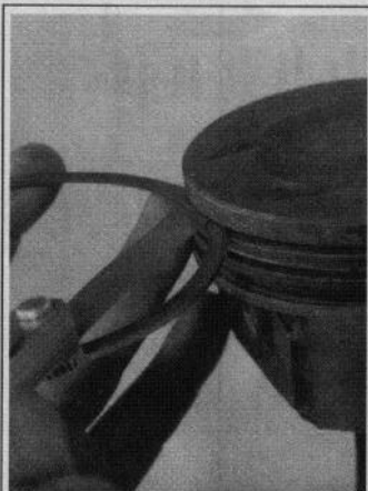
Fig. 269 Checking the piston ring-to-ring groove side clearance using the ring and a feeler gauge
