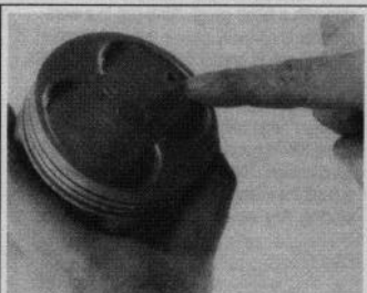
Fig. 264 Most pistons are marked to indicate positioning in the engine (usually a mark means the side facing the front)
