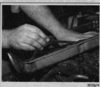
Fig. 11 Remove the valve cover gasket, thoroughly clean the valve cover and cylinder head, and replace the gasket
