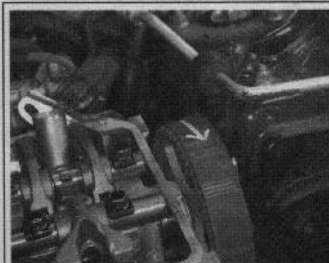
Fig. 171 Make sure you mark the rotation of the timing belt if you plan on reusing the belt
