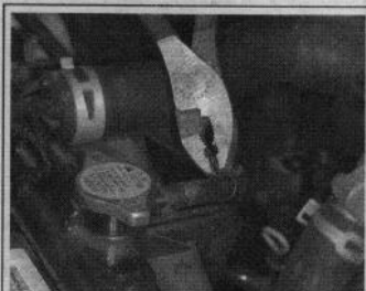
Fig. 77 Use a pair of pliers to remove the hose clamp . . .
