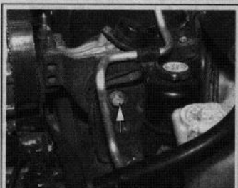
Fig. 165 Remove the upper engine mount through-bolt . . .
