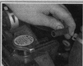
Fig. 78 . . . then disconnect the overflow hose from the radiator
