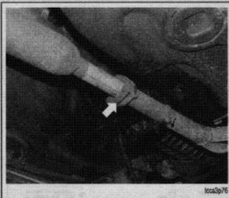
Fig. 222 Some systems, like this one, use large O-rings (doughnuts) in between the flanges
