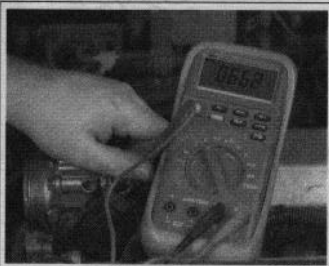
Fig. 72 Testing the SIG RTN circuit of the TP sensor
