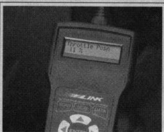
Fig. 74 The TP sensor can be monitored with an appropriate and Data-stream capable scan tool
