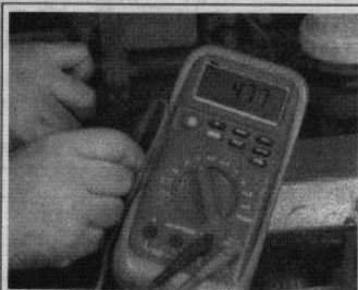
Fig. 71 Testing the SIG circuit to the TP sensor
