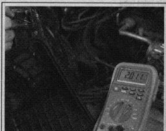
Fig. 54 Testing the resistance of the IAT sensor across the two sensor pins
