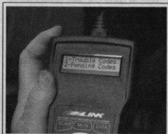
Fig. 90 In this case, we would choose 1-Trouble Codes to retrieve the DTC's
