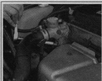
Fig. 50 Use a deep socket and an extension to reach the ECT sensor . . .
