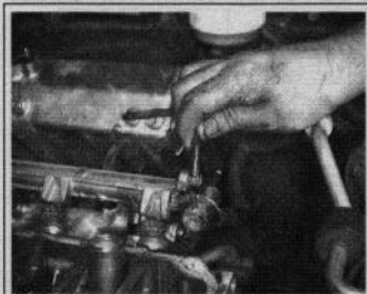
Fig. 25 Remove the vacuum hose from the pressure regulator
