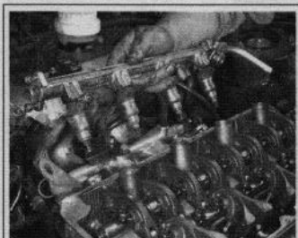
Fig. 28 . . . then lift the rail and the injectors from the intake manifold
