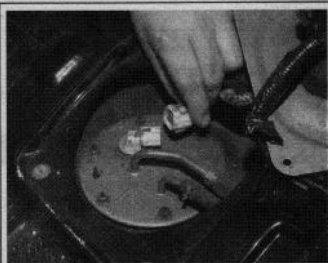
Fig. 69 Detach the electrical connector from the fuel pump
