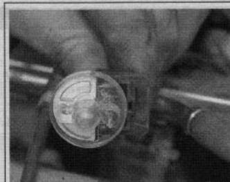
Fig. 36 If the correct "noid" light flashes while the engine is running, the injector driver circuit inside the PCM is working
