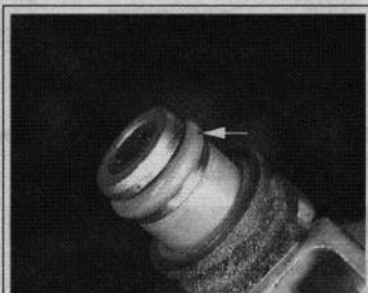
Fig. 30 Always replace the O-rings on the injectors before reinstalling them
