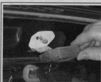
Fig. 111 . . . then lower the lens to access the bulb
