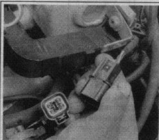
Fig. 6 Weatherproof connectors are most commonly used in the engine compartment or where the connector is exposed to the elements
