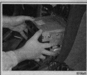
Fig. 37 . . . then slide the radio chassis and bracket out of the instrument panel
