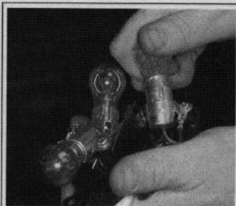
Fig. 108 Rotate the bulb assembly. . .
