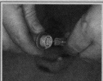
Fig. 104 Pull the bulb assembly straight out of the socket to remove
