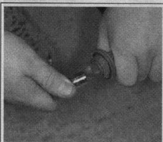
Fig. 93 Pull the bulb assembly out of the socket to remove
