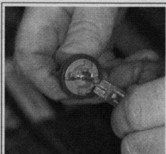
Fig. 89 Pull the bulb assembly out of the socket to remove
