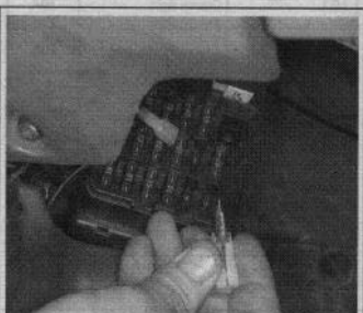
Fig. 126 Grasp the fuse with the removal tool and pull it straight out to remove it
