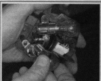
Fig. 97 Depress and turn the bulb assembly, then pull it out of the socket to remove
