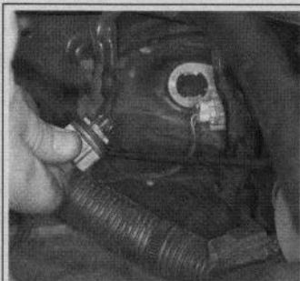
Fig. 88 Twist the bulb socket to release it from the lens
