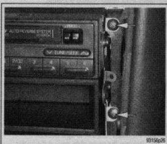
Fig. 36 Remove the radio retaining screws (two per side) . . .
