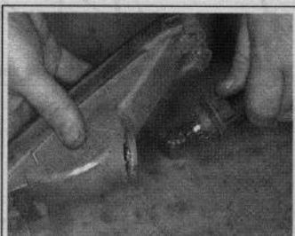
Fig. 92 Twist the bulb socket to release it from the lens
