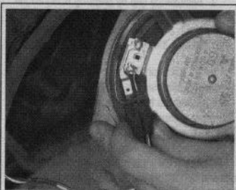
Fig. 52 . . . then detach the connector from the back of the speaker
