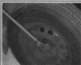
Fig. 1 With the vehicle still on the ground, break the lug nuts loose
