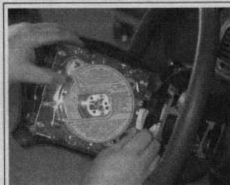
Fig. 79 . . . then detach the connector and remove the air bag module from the vehicle
