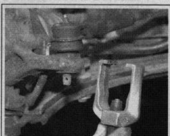
Fig. 88 A special puller is recommended for removing the tie rod end from the steering knuckle without damaging the tie rod end
