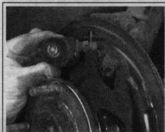
Fig. 98 . . . then remove the wheel cylinder from the backing plate
