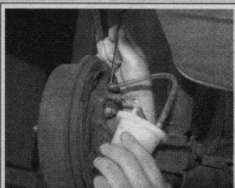
Fig. 26 Slowly open the bleed screw and have an assistant depress the brake pedal while observing the hose for bubbles
