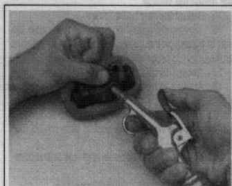
Fig. 100 Compressed air can be used to remove the pistons and seals
