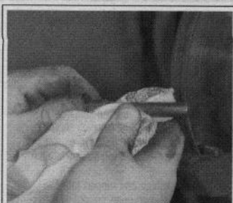
Fig. 41 Thoroughly clean the caliper slides . . .
