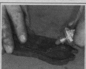
Fig. 47 Apply more brake quiet over the outside of the shim before installing the pads on the vehicle
