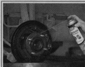
Fig. 93 If a cleaning tub is not available, a quality aerosol cleaning solvent can be used
