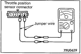
(2) Connect an ohmmeter between terminal 3 (Idle position switch) and 4 (sensor earth) by using jumper wires.
