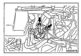
(3) Hold the fuel filter with a spanner and remove the eye bolt. Then remove the high-pressure fuel hose.
