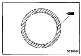
(4) Apply specified sealant to the contact surfaces of the plug and the floor pan, and install the plug.
