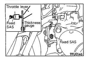
(3) Insert a feeler gauge with a thickness of 0.45 mm (0.0177 in.) between the fixed SAS and the throttle lever.
