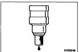
(7) Stop the actuation of the injector, and check for leakage from the injector's nozzle.
