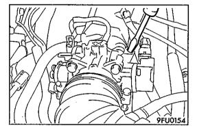
(7) If not within the standard value range, turn the speed adjusting screw (SAS) to make the necessary adjustment. NOTE
