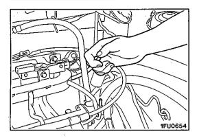
(11)Disconnect the vacuum hose from the fuel pressure regulator and measure fuel pressure with the hose end closed by a finger.
