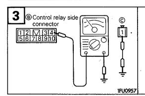
Check for open-circuit or short-circuit between the fuel pump and the fuel pump drive terminal.
