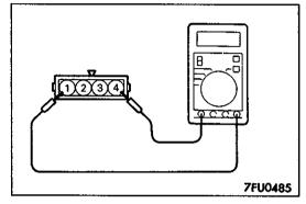
(2) Measure the resistance between the throttle position sensor side connector terminal ① and terminal ④.
