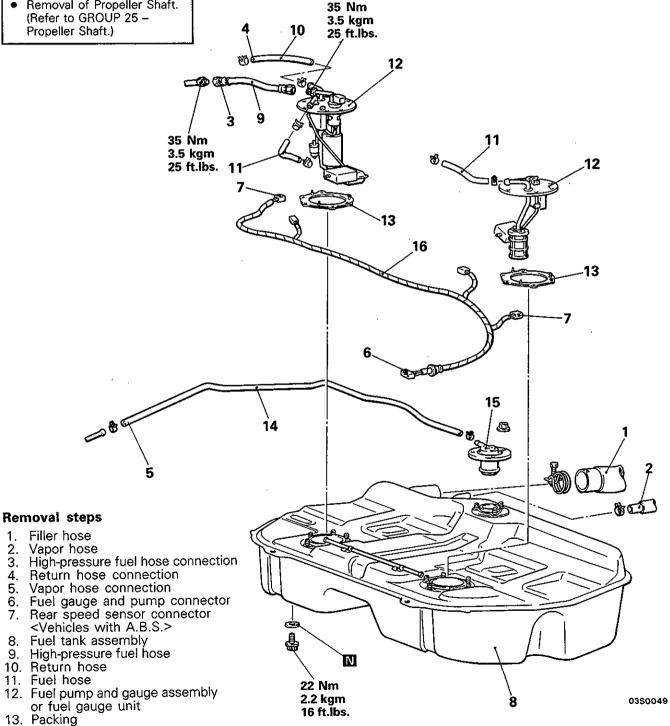
16. Fuel gauge and pump wiring harness
