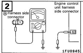
Check for open-circuit, or short-circuit to earth between coolant temperature sensor and engine control unit.
