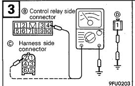
Check for open-circuit or short-circuit between the fuel pump and the fuel pump drive terminal.
