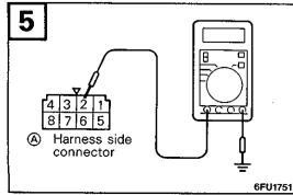
Measure the power voltage to the actuator.
