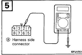
Measure the power voltage to the actuator.
