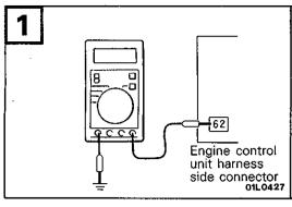
Measure the ignition switch terminal input voltage.
