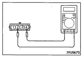
(3) Measure the resistance between the throttle position sensor side connector terminal (2) and terminal (4).
