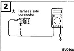
Measure the power supply voltage of the control relay.
