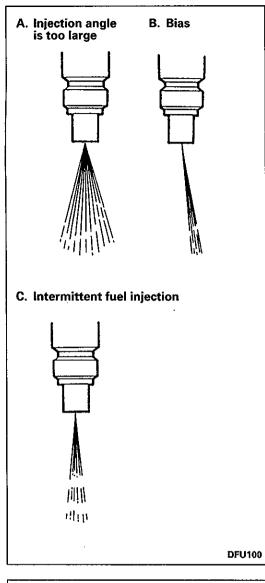
(4) If the fuel injection initial pressure is outside the standard value, disassemble the nozzle holder to clean it, and then change the thickness of the shim to adjust the fuel injection initial pressure.
