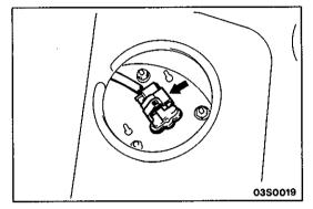
(3) Disconnect the fuel gauge unit connector and remove the fuel gauge unit.
