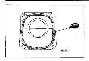
(5) For vehicles with 4WD (except Wagon), after attaching the specified sealant to the inspection lid in the places shown in the illustration, install the inspection lid to the floor.
