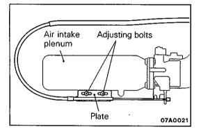
2 Loosen the adjusting bolts on the air intake plenum, and then secure the outer cable so that the free play of the inner cable will be the standard value.
