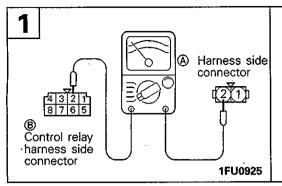
Check for continuity between air by-pass control solenoid valve and control relay.
