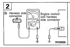
Check for open-circuit or short-circuit between air by-pass control solenoid valve and engine control unit.
