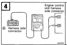
Check for open-circuit, or short-circuit to earth, between the engine control unit and the control realy.
