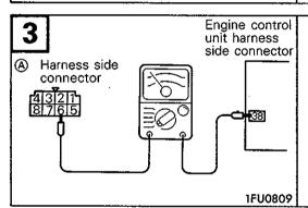
Check for open-circuit, or short-circuit to earth, between the engine control unit and the control relay.
