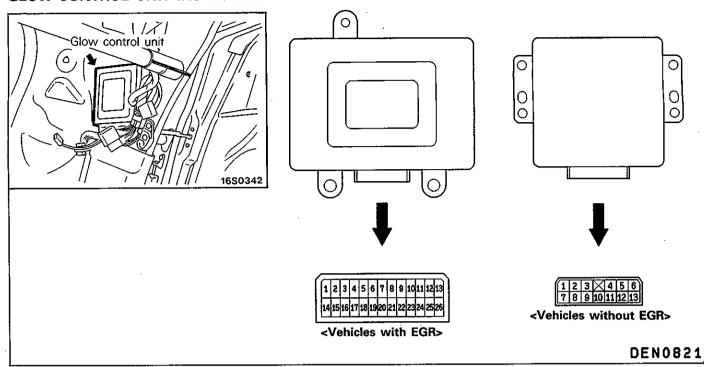
(1) Measure the voltage at the control unit terminals.
