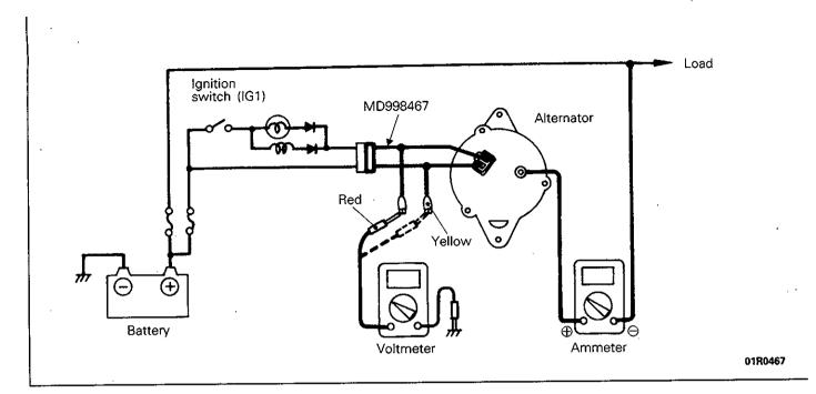
This test determines whether the voltage regulator is correctly controlling the alternator output voltage.
