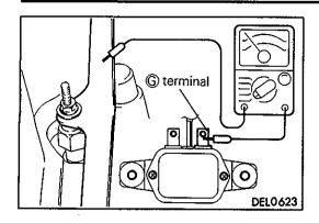
(4) Measure the resistance between the (G) terminal of glow plug relay 2 and the glow plug plate.
