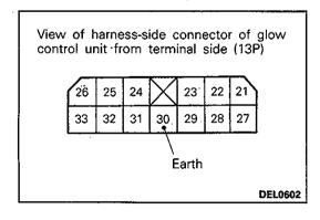
(2) Remove the control unit connector and check the continuity between the harness-side connector terminals.
