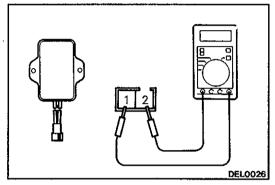
(2) Measure the resistance between the dropping resistor
