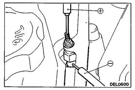
(3) Measure the resistance between the glow plug plate and the glow plug body (earth).
