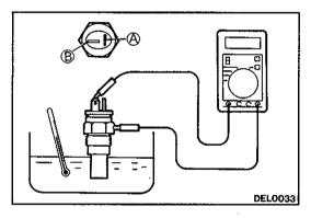
(2) While the sensor section of the engine coolant temperature sensor is submerged, measure the resistance between (B) terminal and the body.
