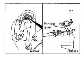
(4) Rotate the adjusting nut to adjust the parking brake stroke to the standard value. After making adjustment, check to ensure that there is no looseness between the adjusting nut and parking brake lever.
