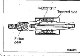
(2) Apply specified fluid to the oil seal inner surface and the O-ring.
