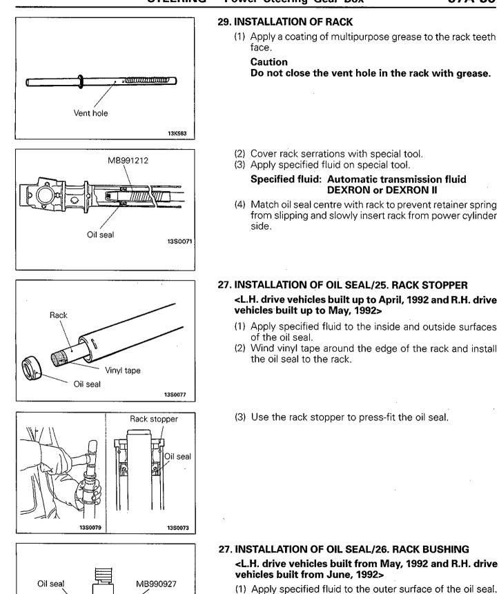
Press-fit the oil seal using the special tool until it is flush with the bushing end face.
