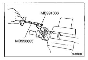
(2) In neutral position, rotate pinion shaft clockwise one turn/4-6 seconds with special tool. Return rack support cover 30°-60° and adjust torque to the standard value.
