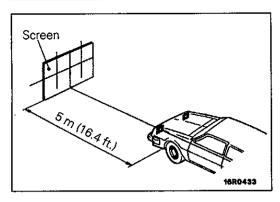
4. Set the distance between the screen and the centre of the fog lamps at 5 m (16.4 ft.).
