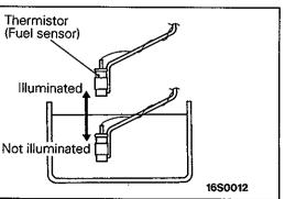
(2) Condition good if light goes off when unit thermistor is in water and lights when unit is removed from water.
