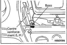
(2) Remove the heater control assembly boss from the center reinforcement (L.H.).
