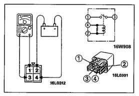
(2) Apply battery voltage to terminal @, and check the continuity between the terminals when terminal @ is earthed.
