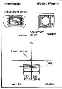
6. Check if the beam shining onto the screen is at the standard value.
