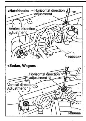
(6) Alternately turn the adjusting screw to adjust the headlamp aiming.
