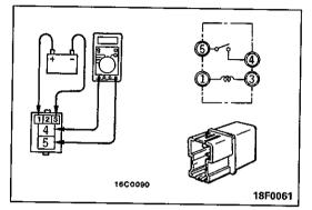
(2) Apply battery voltage to terminal ①, and check the continuity between the terminals when terminal 3 is earthed.
