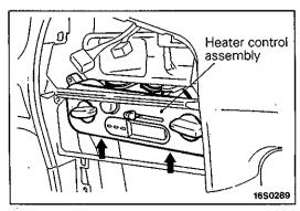
(3) Push the heater control assembly into the instrument panel, remove the clock mounting screws, and remove the clock.
