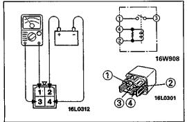
(2) Apply battery voltage to terminal ②, and check the continuity between the terminals when terminal ④ is earthed.
