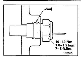
(2) After checking, apply the specified adhesive around the thread of engine coolant temperature gauge unit and install on the intake manifold.
