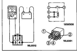
(3) Apply battery voltage to terminal @, and check the continuity between the terminals when terminal @ is earthed.
