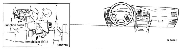
NOTE For R.H. drive vehicles, part installation position are symmetrical.
