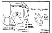
Install a new drain plug gasket so that it faces in the direction shown in the illustration, and then tighten the drain plug to the specified torque.
