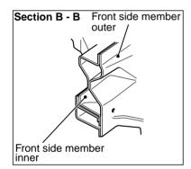
The octagonal cross section for the front of the front sidemember and 8-shaped cross section for the rear of the front sidemember have been adopted for enlargement so that the applied structures can effectively absorb energy from the impact at the time of collision. 2. Due to the adoption of straightened front sidemember and the rear floor sidemember, the structure can effectively absorb energy from the impact at the time of collision.
