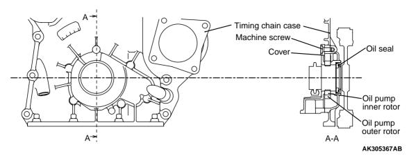
The oil pump is of a cycloid type, directly driven by the crankshaft.
