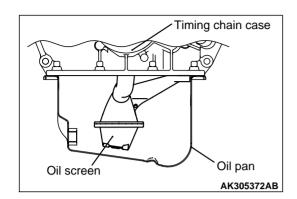
The oil screen is located in the position with the least disturbance to the oil suction volume that results from oil level variation in the oil pan while the vehicle is driven.
